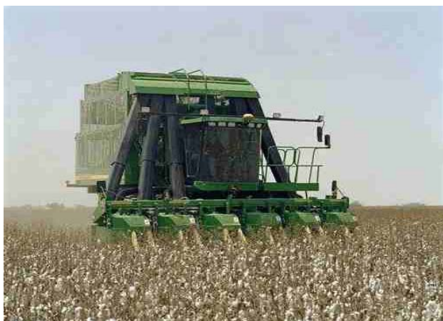
Figure 2.1: Typical spindle-type mechanical harvester for cotton
