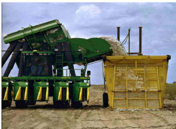
Figure 2.4: Spindle picker dumping into a module builder
