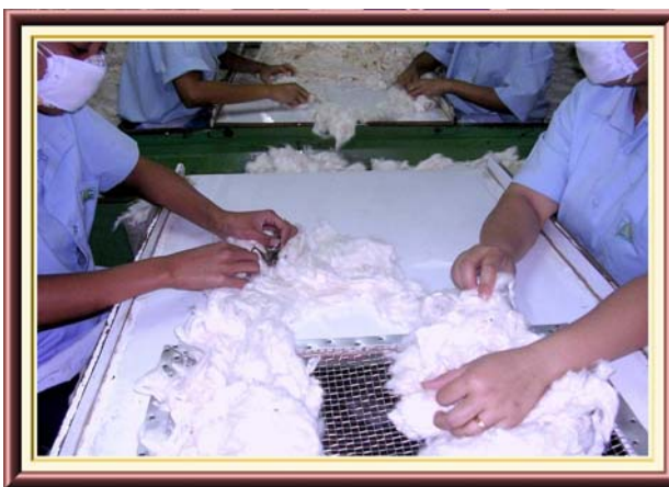
Figure 2.21: Cleaning table with wire mesh and white top
